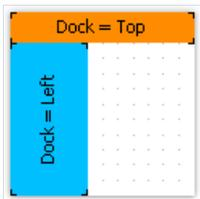
As seen, the height of the second object is equal to height of the free space, which remains after docking the first object.
