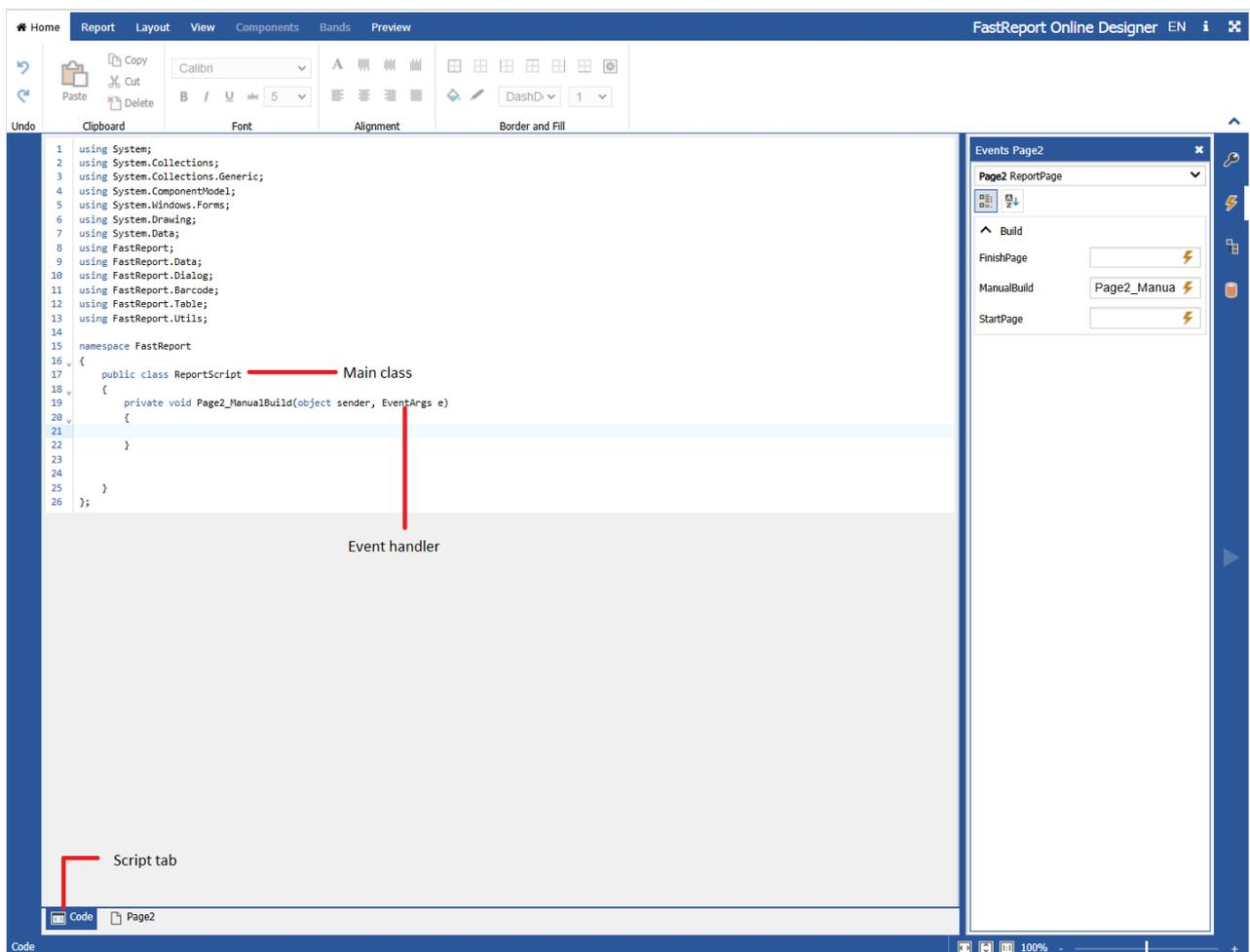
In the figure you can see the "Events" window for the object Page1. This window allows you to create event handlers for components and bands.
