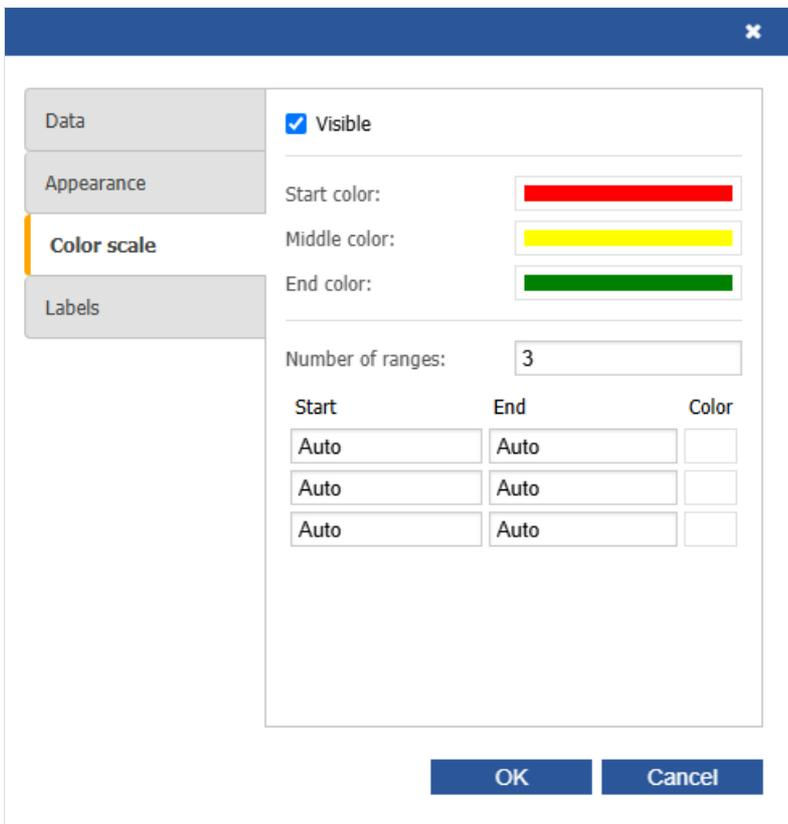
By default all range properties are set to `Auto`, meaning FastReport calculates the minimum and maximum values for each range automatically. The auto color is chosen from three presets ("Start color", "Middle color", "End color"). The `Auto` mode may be suitable in most cases.
