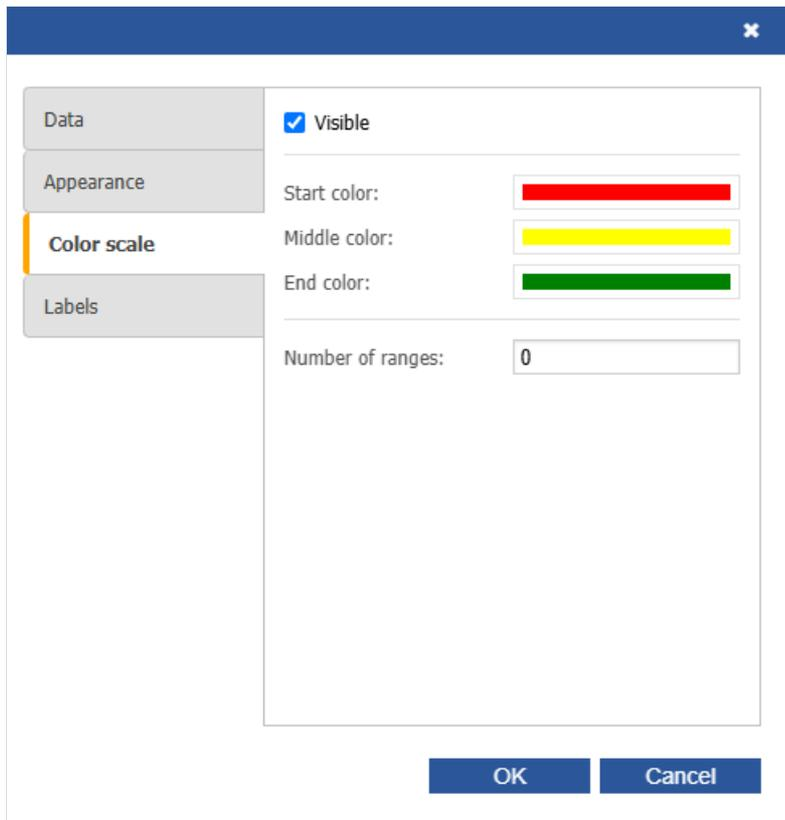
The color scale consists of several ranges. Each range has the following properties: min value, max value and color. You can use as many ranges as you need. To set up the color scale set the number of ranges first and then the properties for each range.
