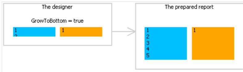
This is needed when printing information in a table form. In a table row there can be several objects which can stretch. This property makes it possible to set all objects' height to the maximum height of the band.
