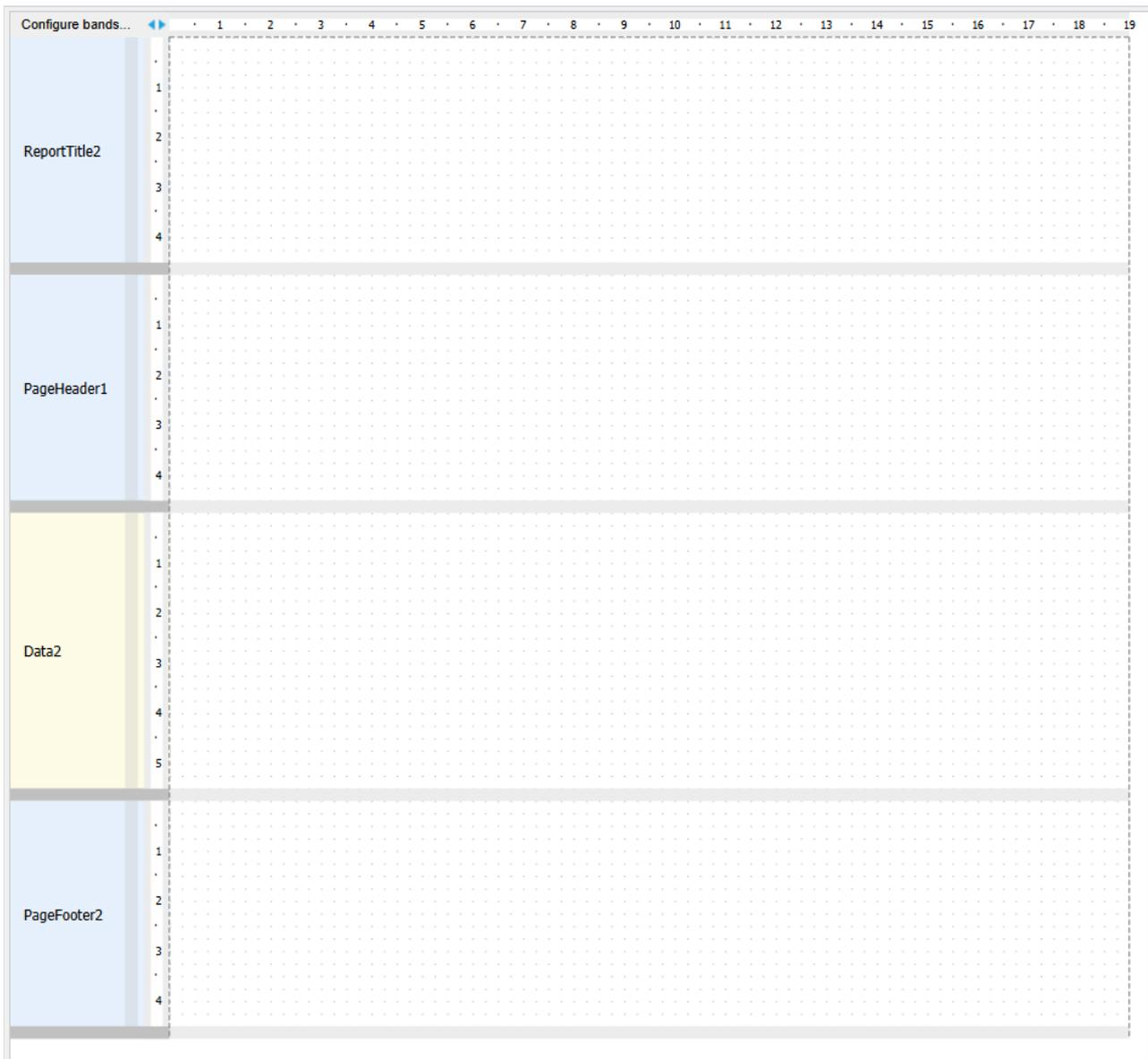
Bands can have a fill and border (disabled by default). Also, bands have a grid displayed in design-time for easy positioning of components. The grid can be set in "View" menu of the main menu.
