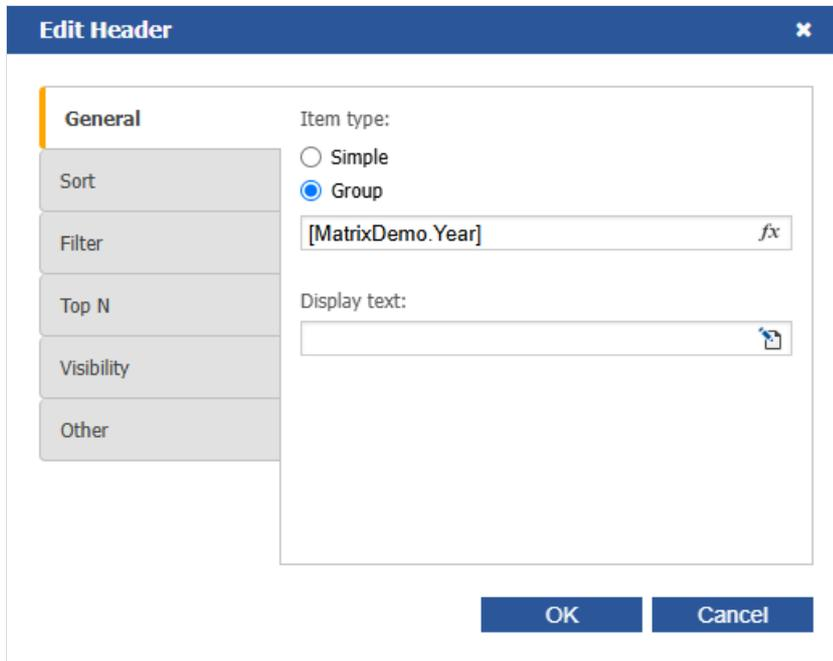
You can turn a simple element into a group and vice versa. Some of the settings in the editor window are not available for a simple element.
