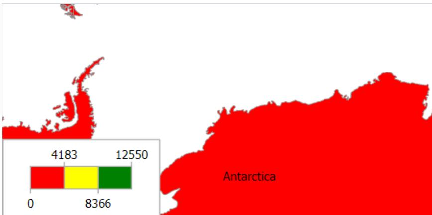
To set the appearance and position of the indicator, select the "Map" element in the layers tree control and switch to the "Color scale" tab:
