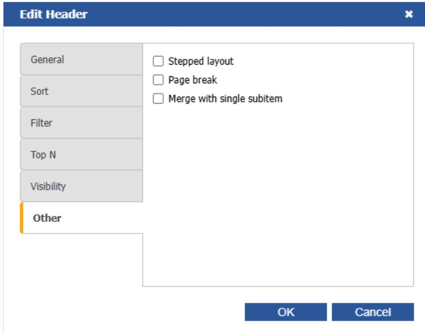
The "Stepped layout" option toggles the layout of nested elements between block (default) and stepped layout. Let's look at the example of a matrix with a nested row header (Year, Month). The block layout looks like this: The finished report looks like this:
