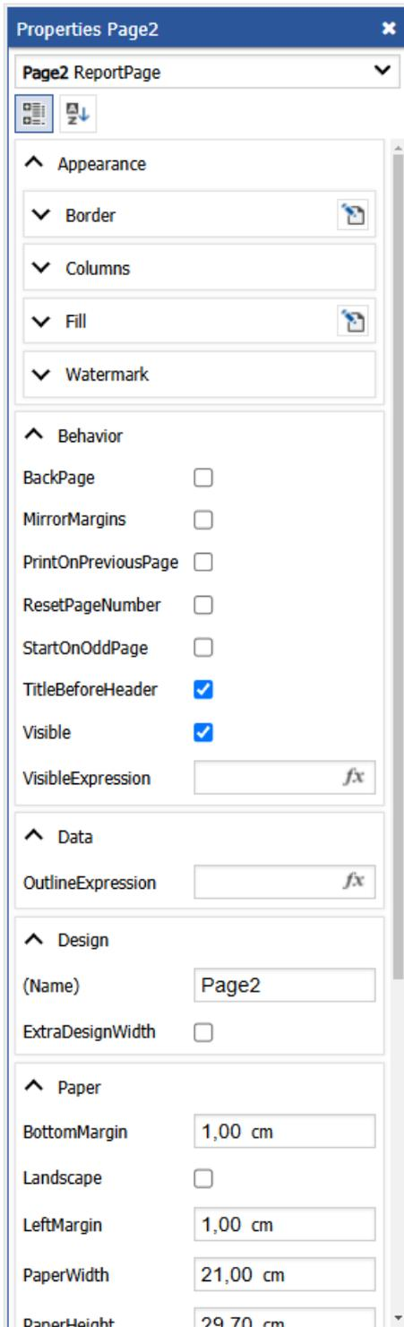
You can set the page size and margins in the "Paper" section. Section "Print" allows you to determine two-sided printing, the source of the first page and the source of other pages. In addition, you have access to the page appearance properties such as border, fill, etc.
