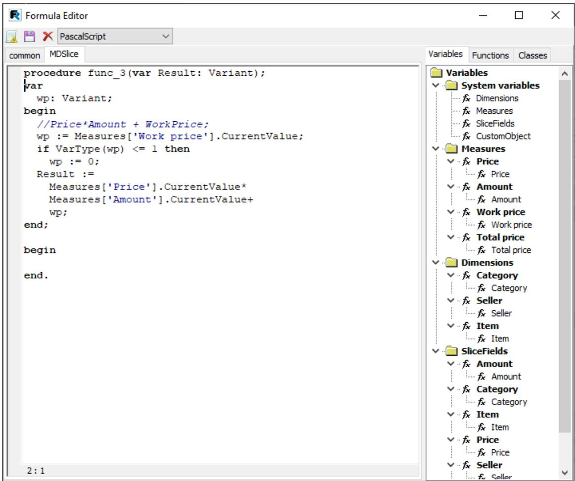
A function which calculates the measure value on other measures is called once for each cell (dimension intersection). If "Calc all cells" is not set then the function is not called for empty cells.
