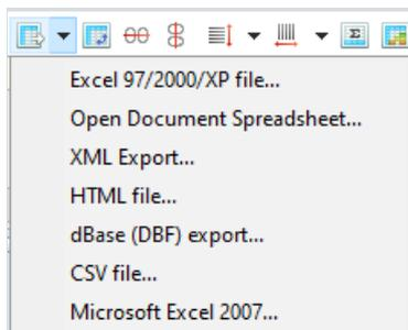
Exporting uses either the grid data or the source cube data, depending on the export format chosen. So, for example, Excel export uses the dimensions and measures in the grid, while DBF export is from the source cube data.
